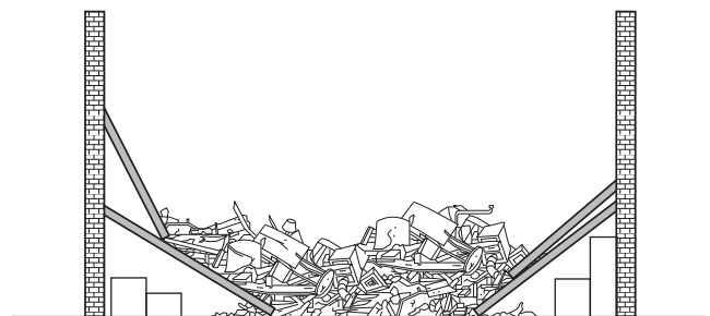
FIGURE D.2(j) Fire Burn-Out Collapse Pattern — Roof/Floor Burn-Out — Heavy Wall Construction — URM or Tilt-Up.
