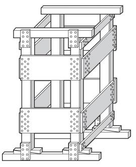
FIGURE A.6.4.3(6)(b) Plywood Laced Post Shore.
