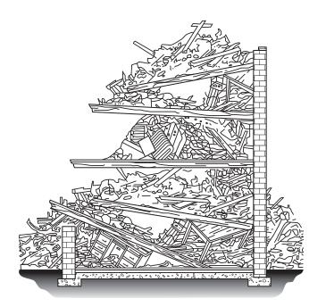
FIGURE I.1(d) Cantilever Floor Collapse. (Courtesy of U.S. Department of Civil Defense)
