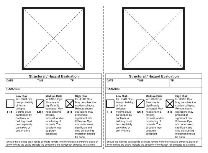
FIGURE F.3.1 Structure/Hazards Placard.
