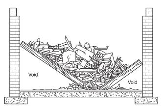
FIGURE I.1(b) V-Shape Floor Collapse. (Courtesy of U.S. Department of Civil Defense)
