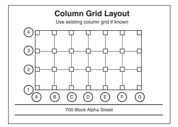
FIGURE F.2(e) Structure Identification Marking System Within a Geographic Area — Column Grid Layout.
