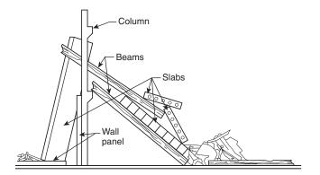
FIGURE I.2(g) Random Fall Collapse Pattern — Precast Concrete Construction.
