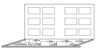
FIGURE I.2(a) Offset Collapse Pattern — Light Frame Construction.
