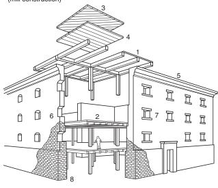
Details: 5. Typical unbraced parapet
