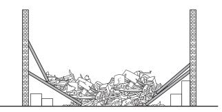
FIGURE I.2(j) Fire Burn-Out Collapse Pattern — Roof/ Floor Burn-Out — Heavy Wall Construction — URM or Tilt-Up.
