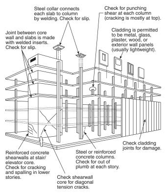
FIGURE C.1(b) Post-Tensioned Lift Slab Building.
