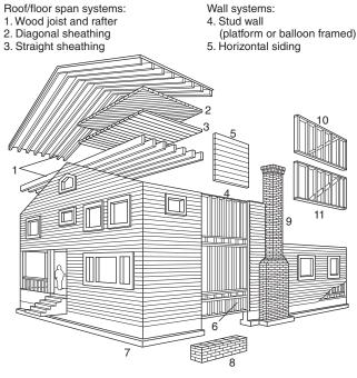
Foundation/connections: 6. Unbraced cripple wall 7. Concrete foundation 8. Brick foundation Bracing and details: 9. Unreinforced brick chimney 10. Diagonal blocking 11. Let-in brace (only in later vintages)
