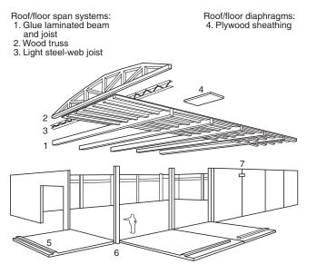
Details: 5. Anchor-bolted wooden ledger for roof/floor support
