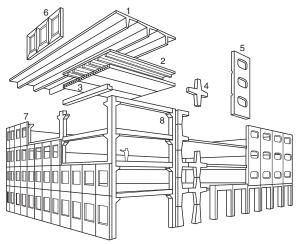
Curtain wall system: 6. Precast concrete panels 7. Metal, glass, or stone panels Structural system: 8. Precast column and beams
