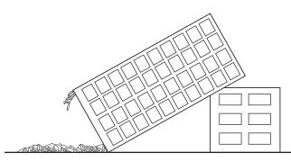
**FIGURE I.2(e)** Overturn Collapse Pattern — Heavy Floor or Heavy Steel Construction.
