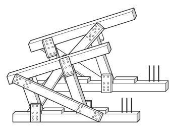
FIGURE A.6.4.3(6)(c) Sloped Floor Shore Type 2.
