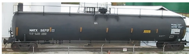
This is an example of a pressure tank car. (Source: Provided by members of the Association of American Railroads)
