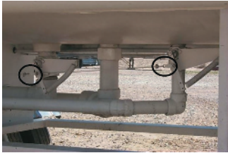
This is an example of a fusible link assembly. (Courtesy of Charlie Wright)
