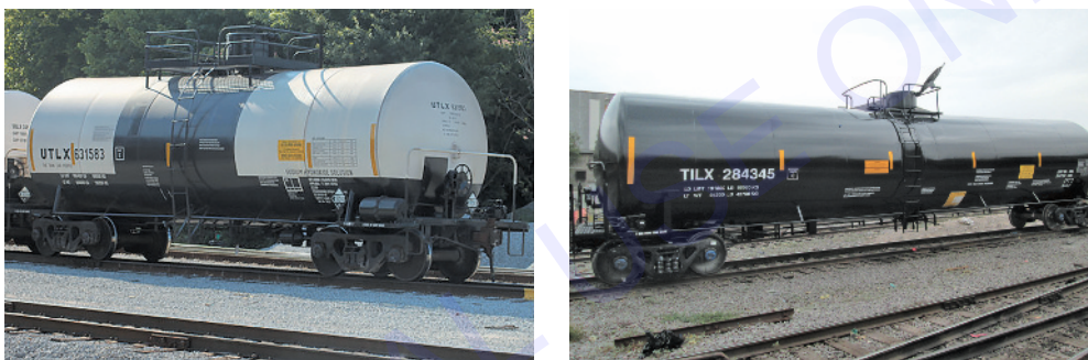
These are two examples of nonpressure tank cars. (Source: Provided by members of the Association of American Railroads)
