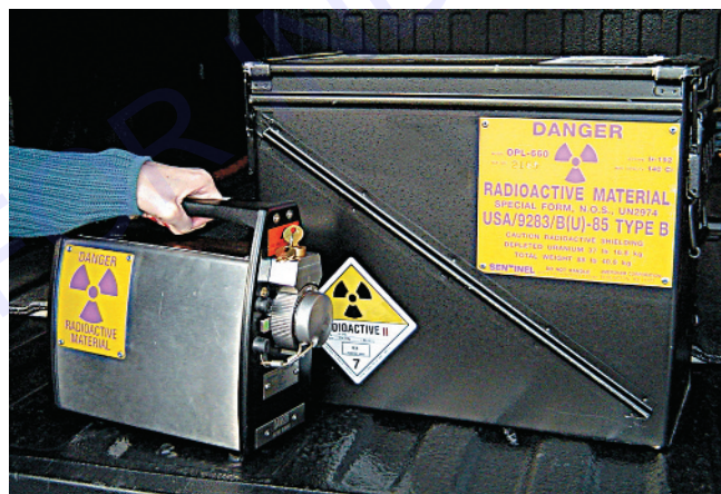
Examples of radioactive materials packaging Type A and Type B: Radiopharmaceuticals are commonly transported in Type A packages resembling the ones pictured (left). Type B packages can range from small handheld radiography cameras similar to the one shown (right) to heavily shielded steel casks that weigh well over 100 tons.
