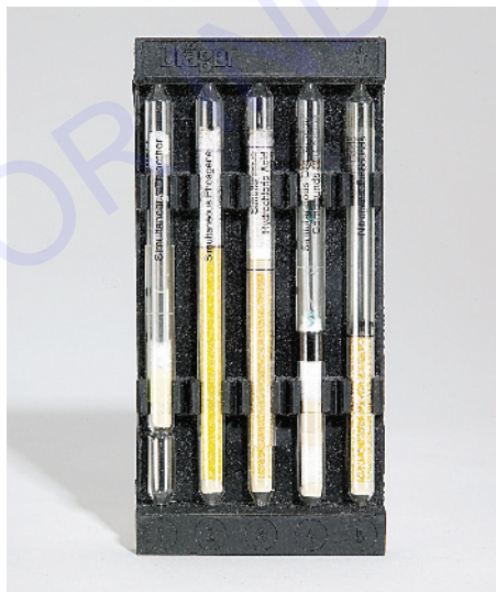
Colorimetric detector tubes are glass sampling tubes used to test for specific toxic materials. (Courtesy of Draeger Safety, Inc.)
