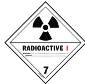
Example of a Radioactive White I label. (Source: Department of Energy Transportation Emergency Preparedness Program)
