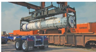
This is an example of an intermodal tank changing modes. (Source: Provided by members of the Association of American Railroads)
