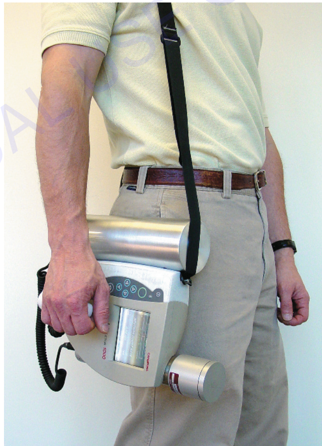
Photo shows an example of a neutron detector. (Courtesy of Mirion Technologies, Inc.)
