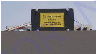
This is an example of a GPS transponder with a yellow label and emergency contact phone number. (Source: Provided by members of the Association of American Railroads)
