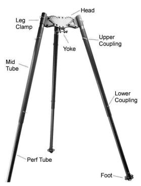
An overview of the head section along with the correct names of each component is presented below. Please refer to this image while learning how to assemble the TerrAdaptor as outline in Section 2.
