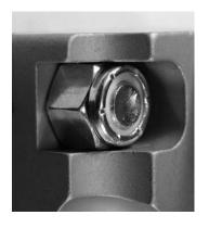
Fig 19 Bolt protrudes just beyond flush
