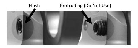
To remove the foot from the adaptor, loosen the piloted screw until the foot is able to slide over the secured pin. It is not necessary to remove the special piloted set screw completely in order to remove the foot from the adaptor.
