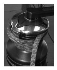
Raise loads by turning the handle in the direction that provides the best mechanical advantage for your situation. Depending on the weight of the load and the speed needed to raise the load, it may be more efficient to place one foot near the base of the tripod leg or lash the leg to the surface for greater stability. Note that the winch can be rigged for progress capture by attaching prussic or other progress capture devices to the rigging points on the winch bracket.
