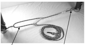
Fig 12 /Rope Hobble Loop with Prussic. Sewn loop connected to quick link; large loop connected to 2<sup>nd</sup> leg quick link.
