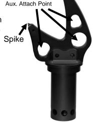
Spikes can be sharpened with a hand file or replaced as they wear. To replace spikes, loosen the small set screws on the side of the Talon points and with hand pliers pull the spikes out from the end. Install new spikes and then tighten the set screws.
