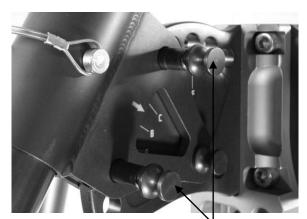
Fig 4 Load Locking Head Pins (Parked position)
